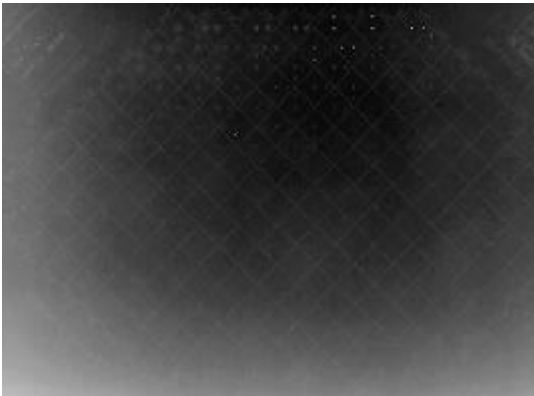
Fig. 2 (a) Analog screen-film CDMAM phantom image. This image was obtained at 25 kVp and 194 mRad mean glandular dose, using a clinical screen-film mammography system, (Model: M-III, LORAD Corporation, Danbury, CT)
